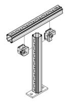
Part List 1x Profile PRO 46-P 1x Cantilever Bracket AK 46-P 2x Angle Connector CN 46
